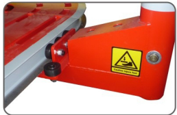
Free moving mechanism of pulling tower
