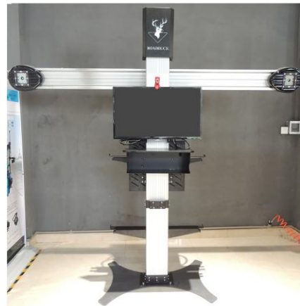
12. Install the 32" LCD and camera
