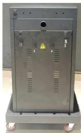
13. Install the back shroud
