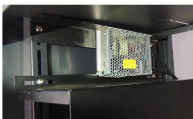
10. Install the standalone power inside the cabinet (between the cabinet rack and the printer bracket)
