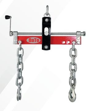
The Engine Leveler is a viable equipment to be used in conjunction with the Engine Crane to position the Engine suitably to fix inside the Engine Room. Providing directional movement by screw and thread the Engine Leveler is a wise choice for easy handling of the Engine with the Engine Crane.
