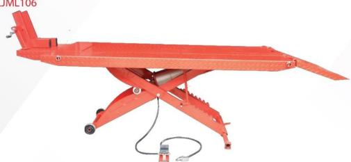
The Most durable and safe operation motor cycle lifts. Designed with Front wheel Locking mechanism to stabilize the Vehicle. DaTo Motor cycle lift works on the Pneumatic Pressure for the hydraulic unit. DaTo Lift is Portable and it also has the
