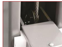
Rack Slope Safety Device The integrated slack rope safety device prevents a tilted position when lowering the platform
