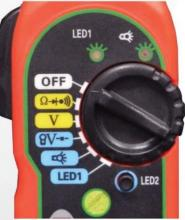
ACT100 is a multi-function circuit testing tool, with the special design of testing probe. This tester can detect various fault locations of the automobile circuit safely and efficiently, without peeling the wire. It can be applicable for the maintenance of automobile circuit, and for the automobile accessories, such as the installation of burglar alarms, sound, GPS anti-theft tracking system, subwoofer, etc.
