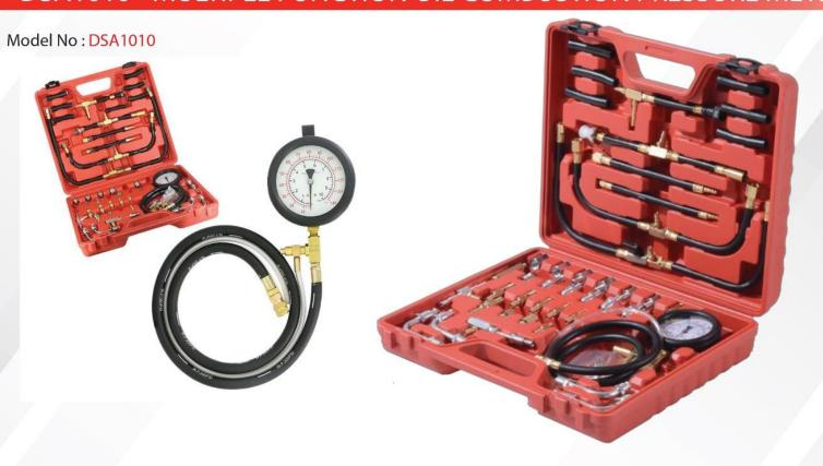
Multiple-function oil combustion pressure meter has a comprehensive kit of adaptors and fittings for most fuel injection system. It has 3-1/2" gauge with dual scale (psi and bar), reading from 0-140 psi and 0-10bar. Hanging hook and protective bumper especially for gauge. Pressure release valve fitted with long drain hose allows safe recovery of pressure and fuel.
