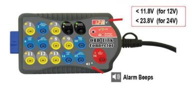
The Pin's LED will blink slow, steady and fast to indicate if there is a presence of voltage (positive or negative) detected at a particular pin. If there is a reverse polarity occurred, the green LEDs at pin 4 (Chassis) and pin 5 (Signal) ground will light up and turns into red color.
