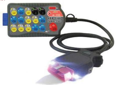
The Innovative OBD Link Connecter performs tests on each and every 16 pins of OBD2 port for abnormality caused by shorting or reverse polarity with ignition key is OFF, ON and engine running to avoid damage to your scan tool prior plug in. - The voltmeter displays voltage input with alarm "Beeps" trigger if voltage falls below 11.8V or higher than 15.2V (for 12 V System) or below 23.8V or higher than 29.2V (for 24V system).
