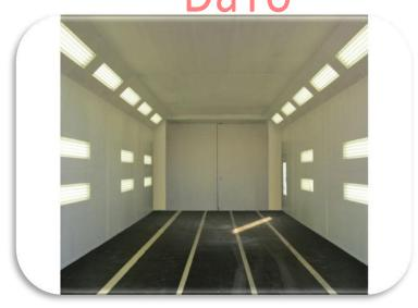
Mid Lights: 4 sets of 40W Tube lights on each side comprising of 160W
