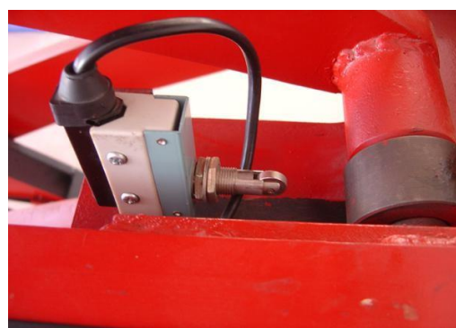
Picture 25(up limit switch of second lift)
