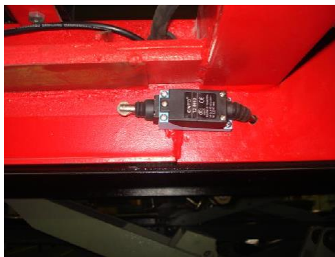
Picture 24(up limit switch of main machine)
